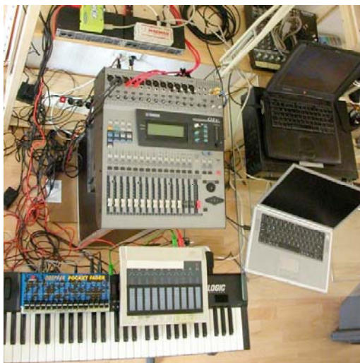
Figure 1. Two laptops, two audio interfaces, a master keyboard, two fader boxes, two MIDI interfaces, a mixer, 8 power supplies, 20+ cables
