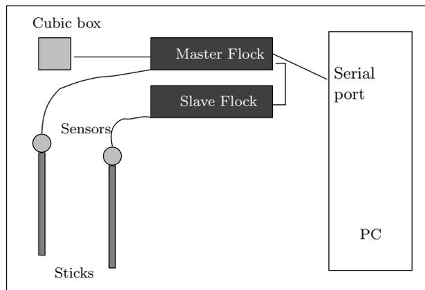
Figure 1: System Architecture for recording and analyze inputs coming from the FOB
