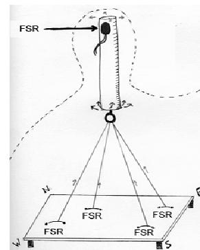
Figure 1. Diagram of internal structure. FSRs mounted below stationary platform.
