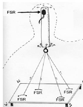
Figure 1. Diagram of internal structure. FSRs mounted below stationary platform.
