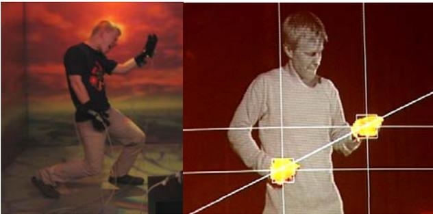
**Figure 4. Left: rocking on with the VR version of the Virtual Air Guitar. Right: computer vision view of the desktop version. A web camera interface tracks the yellow gloves and uses gesture recognition to detect plucks, vibrato, slide and mute.**
