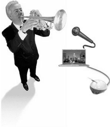
Figure 4. Audio transformation schematics. Pitched audio is detected and segmented by the computer. The Beatbug sends control information to trigger and transform the audio.
