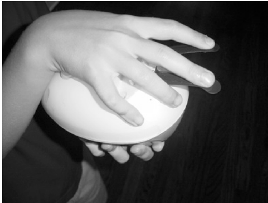
Figure 3. A player taps the Beatbug while bending the antennae to start recording.
