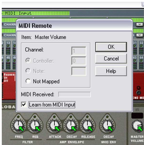
Figure 5: Assigning a MIDI controller to an on-screen control of the Reason GUI.
