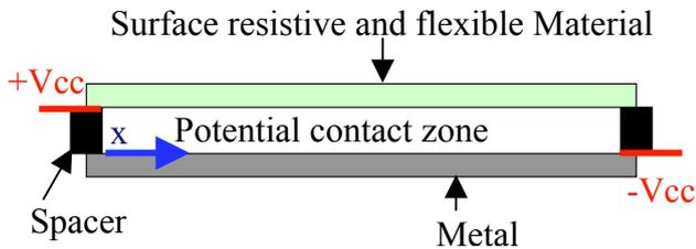
**Figure 2 Home-made linear potentiometer along the x-axis**
