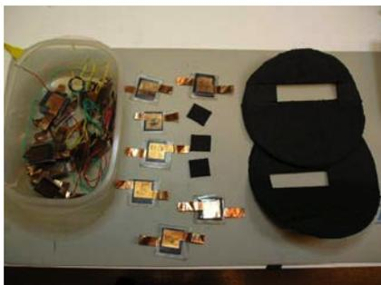
Figure 7 Home-made paper pressure sensors
