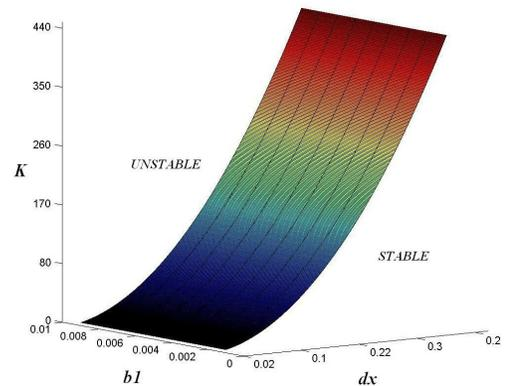
**Figure 4. Stiffness parameter K availability space, resulting from the stability condition.**
