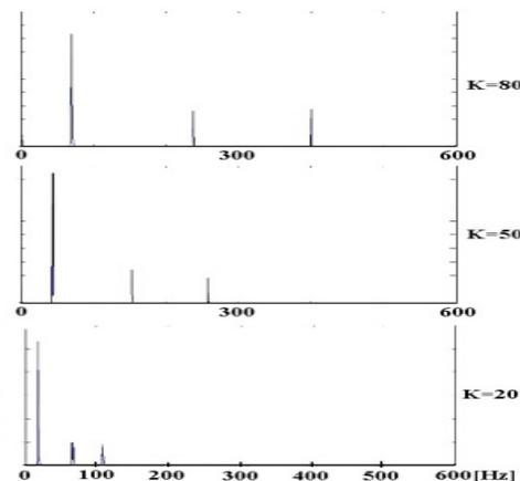
**Figure 5. Spectrum of the produced sound for three different parameters K: 80, 50 and 20**
