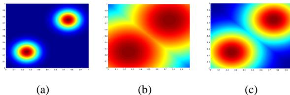
Figure 2. Effect of different values of parameters  $\sigma_{xk}$  and  $\sigma_{yk}$  on 2D Gaussian potential functions
