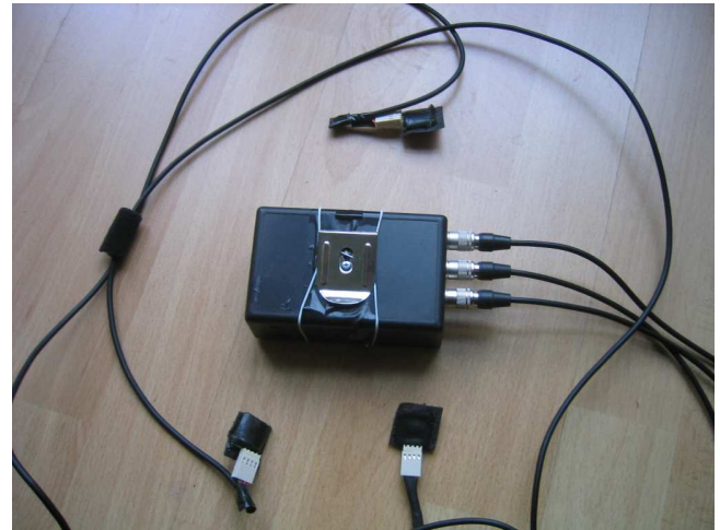
Figure 3: The bodypack, the dancer is wearing. The box is attached to a belt on the waist with the clip. The cables are fixed to his body at certain crucial points (on the chest, on the shoulders and near the elbow) to ensure that the cables stay close to the body, yet have enough slack to move with the body.
