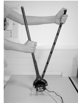
Figure 4. The DAMPER in the "edge-trimmer" configuration.
