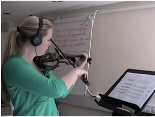
Figure 1: Using the recently created playable measurement system developed in [28] that was evolved from earlier Hyperbow designs, audio and calibrated gesture data are easily collected in simple recording sessions conducted in normal performance environments.
