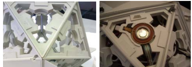
Figure 3: The A20 frame (left) consists of 20 triangles, 16 of which hold flat speakers. Transducer and Force Sensing Resistors (right) fit under each speaker.
