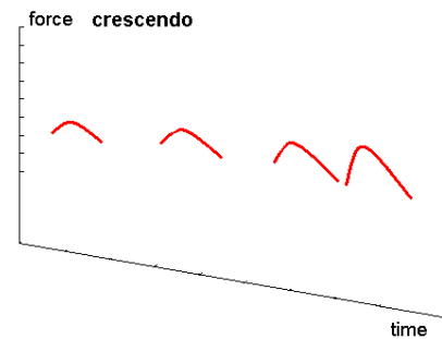
Figure 10. Piano Key Strokes, from “piano” to “forte”, Sensors stuck on the finger tips
