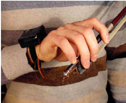
Figure 2. Pressure sensors on the bow
