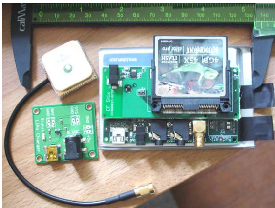
Figure 2. The Gumstix computer with a 4GB Compact Flash Card on top, the battery underneath and both the LiPo charger circuit and the active GPS-antenna on the left.
