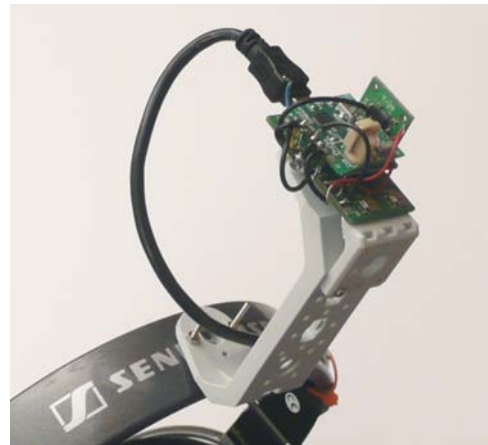
Figure 4: IMU+magnetometer hybrid sensor built on the Bitwacker running uOSC , mounted on Sennheiser HD650
