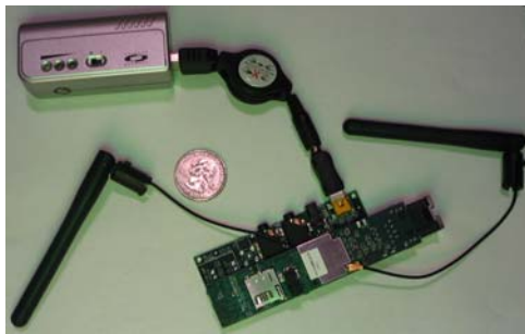
Figure 2: Gumstix size relative to a quarter
