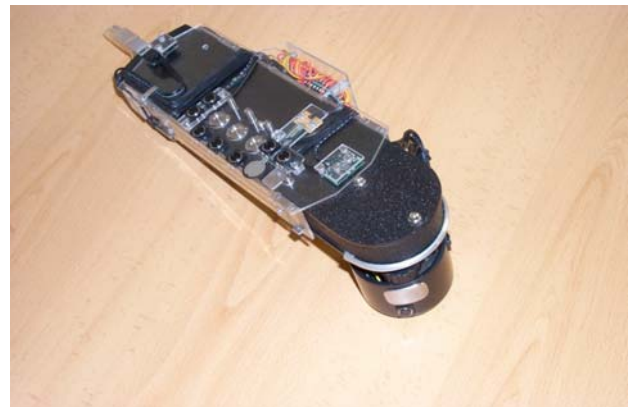
Figure 1. Top view: virtual valves, accelerometer, gyro, FSR
