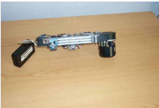
Figure 2. Side view: joystick and 3-membrane sensor
