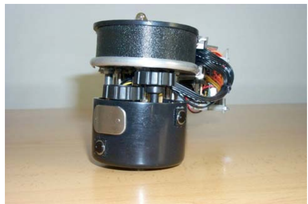
Figure 3. Canister view: 2 potentiometers and 3 switches
