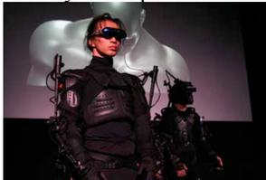
**Fig.2: A movement-registering mechanism built into the BodySuit allows a person's movements to directly control the behavior of an avatar in Second Life.**
