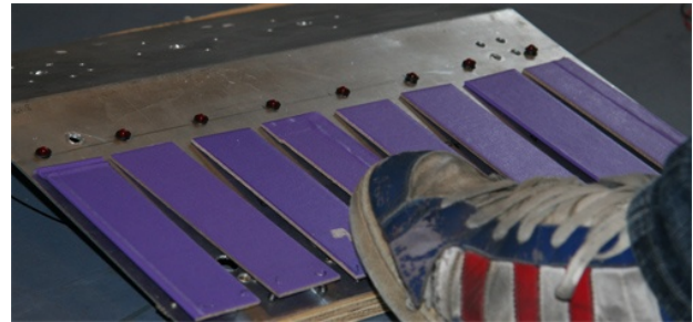
Figure 2: The prototype of the foot-pedal sequencer in action
