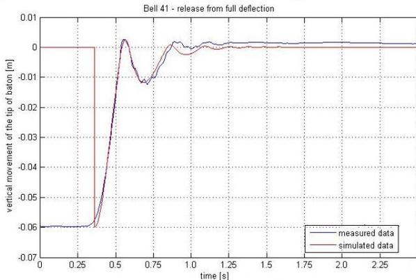
Figure 9. Simulated and measured motion of bell 41
