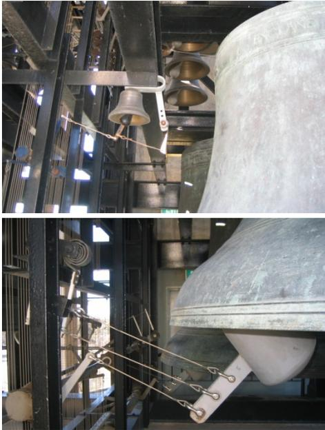
**Figure 1.a (top)** Bell 54 is the small bell (left) shown next to bell 4 (right); note the spiral torsion spring pulling the clapper away from the inside of bell 54. **Figure 1.b (bottom)** also shows bell 4; note the spring pulling the clapper toward bell 4.
