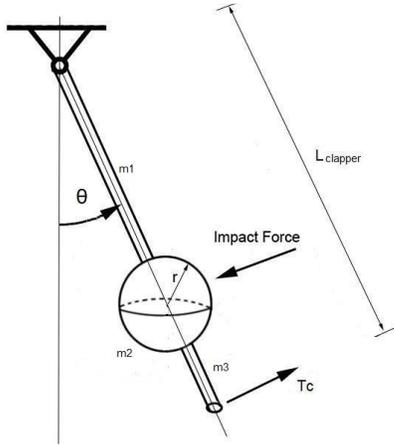
Figure 4. Simplified clapper mechanism.
