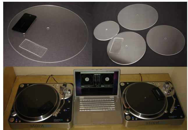
Figure 7: Prototype Hardware. (Upper Left) Phone, plexiglass disc, and sticky rubber. (Upper Right) Various sized and weighted discs to accommodate a performer’s sense of tactility. (Lower) Prototype setup.
