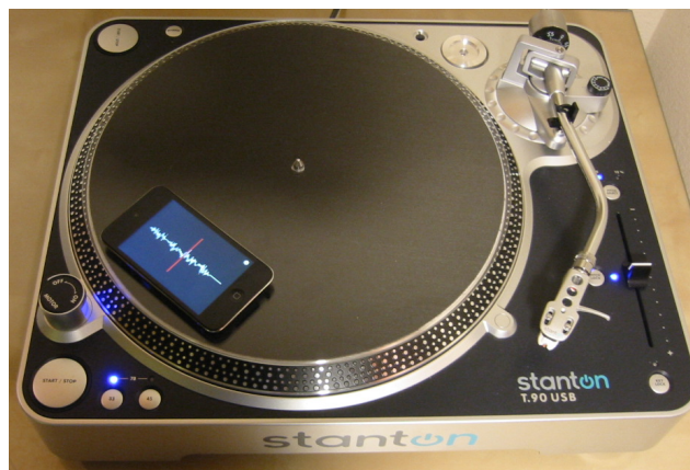
Figure 2: Wireless Sensor Record In Action. A prototype record (combination of mobile phone, sticky rubber, and plexiglass disc) resting on a standard, commercially available turntable.
