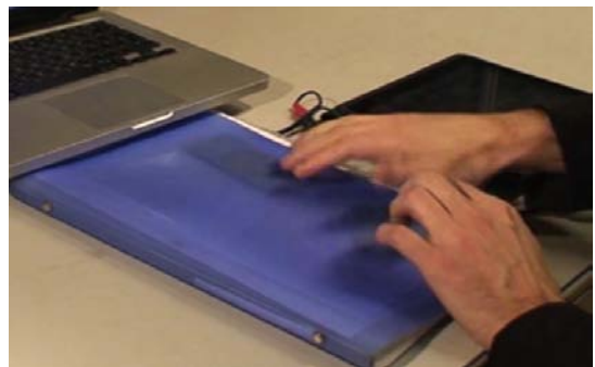
Figure 3: Piezo microphones under a corrugated plastic folder, allowing to hit, scratch, and strum a corpus.
