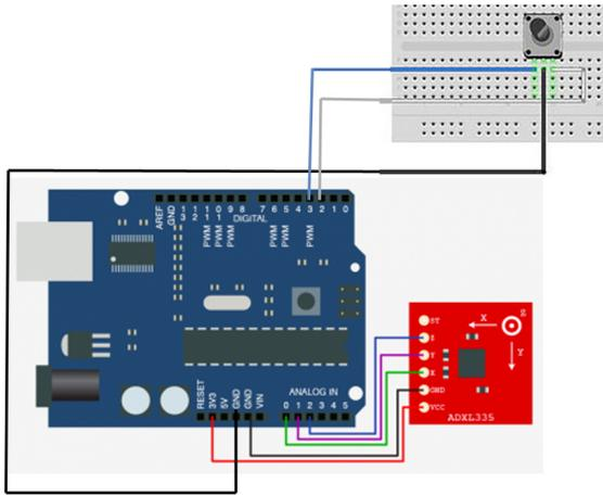
Figure 2: Scheme of sensors' connections
