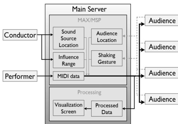
**Figure 2. System diagram of SSN. MAX/MSP was used in order to communicate with performer and audience's devices. Processing language was also used for visualization.**
