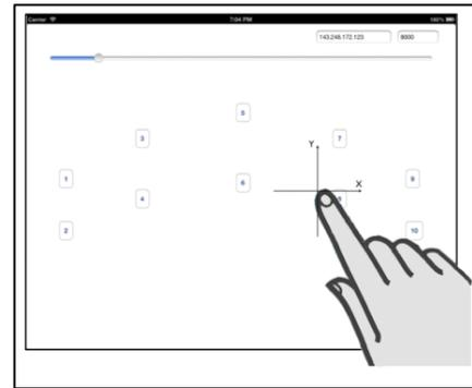
**Figure 3. Performer's app. The performer changes the location of sound source using dragging, and controls the influence range by slider control or pinch gestures**
