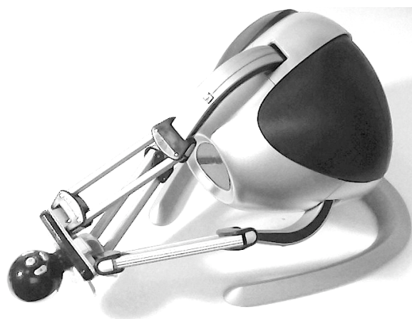
Figure 1. Novint Falcon haptic device, shown with the ball grip on the left-hand side
