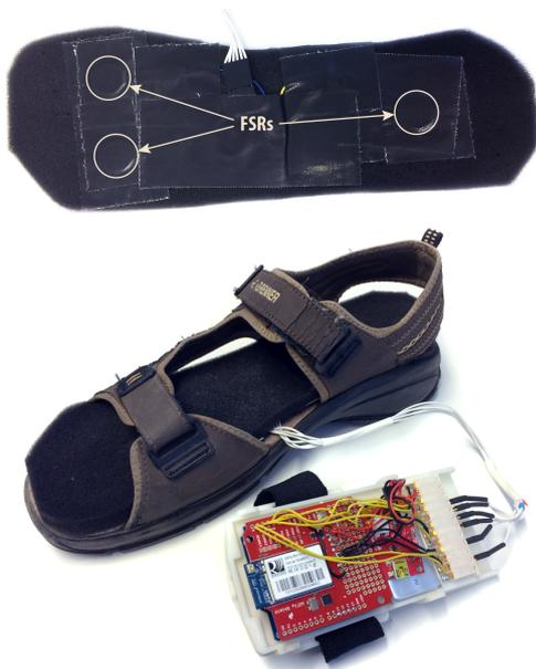
Figure 2: The sensor sole with three force sensitive resistors attached with duct tape (top) and a sandal connected to the GPSP interface with exposed electronics (bottom).
