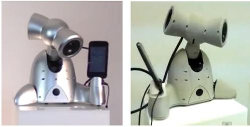
Figure 1: Shimi is a robotic musical companion that employs the “dumb robot, smart phone” approach and engages users with a variety of musical applications.
