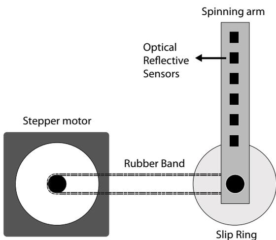
Figure 2: Diagram of Radear's mechanism
