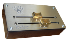
Figure 1: The FireFader open-source hardware haptic force-feedback device.
