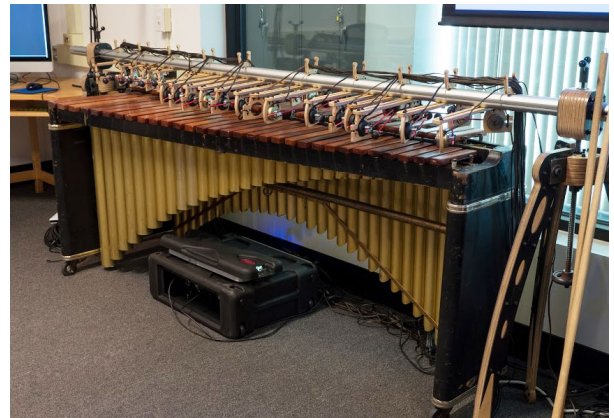
Figure 6: MalletOTon's actuator array positioned above a marimba. The actuators may be repositioned for use with other instruments.
