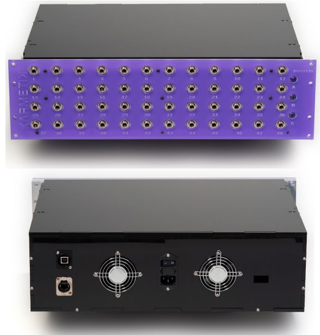
Figure 3: Novalis front and back views. Novalis contains 48 MOSFET drivers to control actuators.
