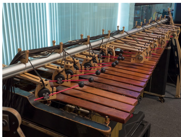
Figure 1: MalletOTon, a new modular and extensible mechatronic mallet instrument player.
