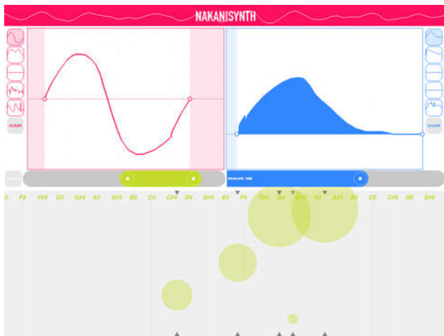
Figure 3: The application’s interface with the ribbon controller option selected, which is shown in the bottom half of the screen. The green circles signify touch events, which increase in size towards the top of the ribbon controller area demonstrate the increase in volume.
