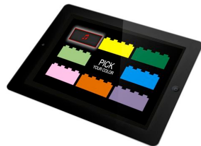
Figure 4. Two iPads were used to connect instruments to the stage. The colors correspond to the color labels on the 8 instruments. In this figure the red instrument is connected to the stage.
