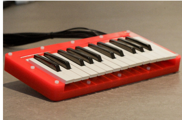
Figure 1. The MRI-compatible keyboard, with fiber-optic cables exiting at the back of the laser cut case.
