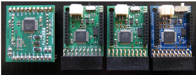
Figure 4: The different hardware revisions of the MiniBee; from left to right revision A, B, D and F.
