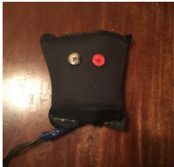
Figure 2: Exhibition prototype – Voice-coil actuator housed in a soft material and sewn shut.
