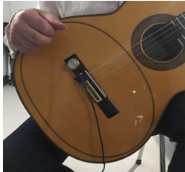
Figure 1: Pickup positioning during recording session. The black oval around the bridge is part of the "membrane" design of the guitar. This highly flexible membrane results in increased volume.
