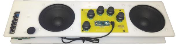
Figure 7: An embedded acoustic instrument for controlling a pair of coupled circle maps as extended with a digital waveguide.
