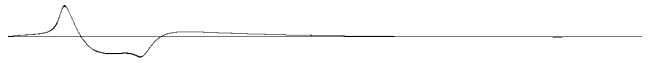
Figure 1: A waveform of a single neuron spike using the Neuron synthesizer (AC-coupled)
