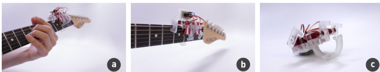
Figure 1: a) Guitar Machine plays alongside a human musician allowing the user to create note combinations that are not accessible, b) consists of robotic fingers of configurable length, c) and press-fits onto the neck of a regular electric guitar.
