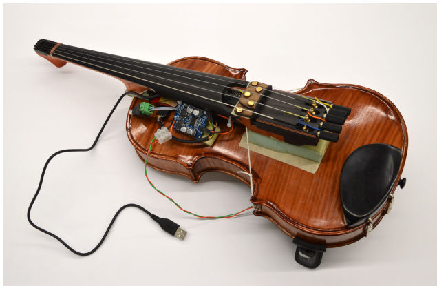
Figure 1: Assembled svampolin with foam separating the stick-violin from the resonating body which is attached upside-down, with the actuator beneath.
