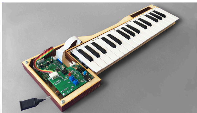
Figure 1: A KeyWI (without cover), including a Bela Mini, custom PCB, enclosure, and sensors
