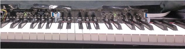
Figure 8: The keyboard scanner installed on the Yamaha CP-300.
