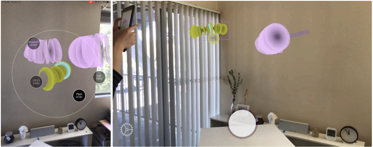
Figure 1: ARLooper multi-user mode. An iPad user’s screen with the multi-touch GUI (left) and an iPhone user’s screen showing the activity of the iPad user (right). In the circles of the multi-touch GUI, the names and values of sound filters are shown. A bounding box around a selected waveform appears in both screens.
