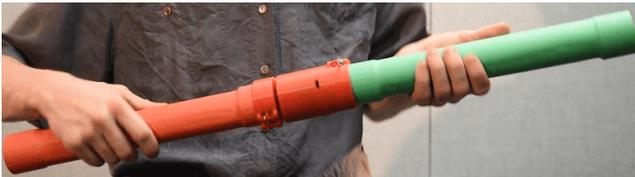
Figure 1: TorqueTuner as a rotary force feedback joint between two T-Sticks
