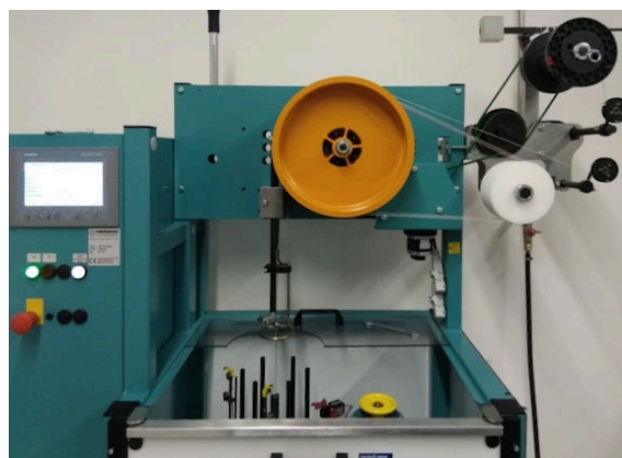
Figure 2: Device for electroding of the fiber.
