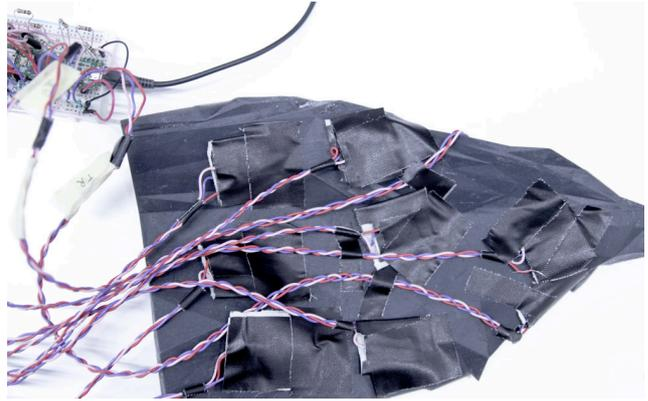
**Figure 2: Pressure pads attached on the inner surface of the instrument**
