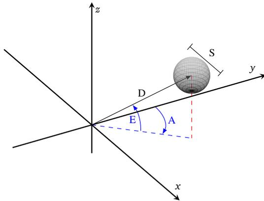
Figure 5: The virtual sound source with controllable parameters.
