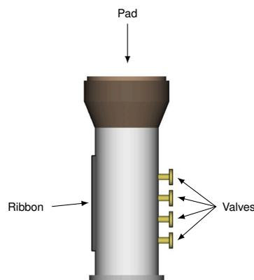
Figure 3: Force-sensing units.
