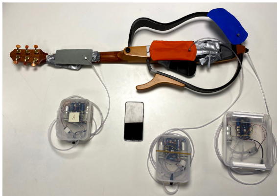
Figure 4. Group 2's breathing guitar concept prototyped through three strategically placed inflatable pads
