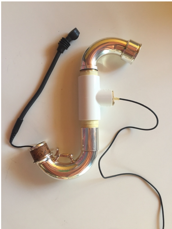
Figure 3: Close-up of the miniature microphone passing through the neck thanks to a plastic joint made from segments of PVC pipe (a T-piece with a lateral segment). The microphone is then plugged with a cylinder of cork.
