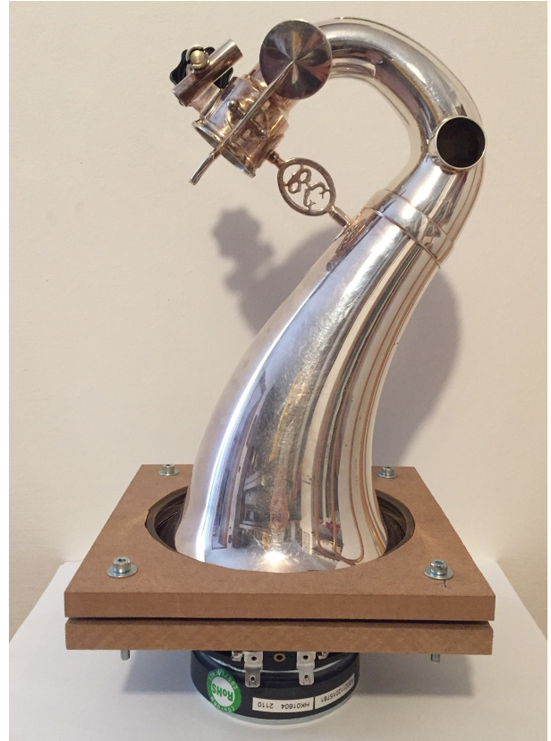
Figure 2: Close-up of the self-made wooden double frame to attach the loudspeaker to the bass clarinet’s bell. The speaker cone is screwed to the first frame, and the internal border of the two frames is lined with foam insulation tape, self-adhesive, to avoid scratches. The two frames are then held together with four screws.
