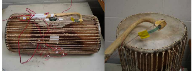
Figure 5. The Lunga with distance (L) and force sensors (R)
