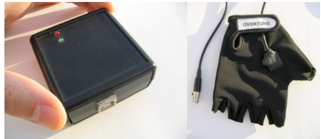
Figure 4. The USB RF receiver and glove with sensors.
